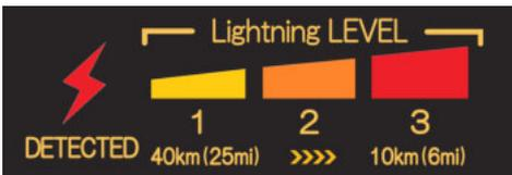
DETECTED : LED lights up in red and issues a beeping alarm when the device detects a lightning strike
